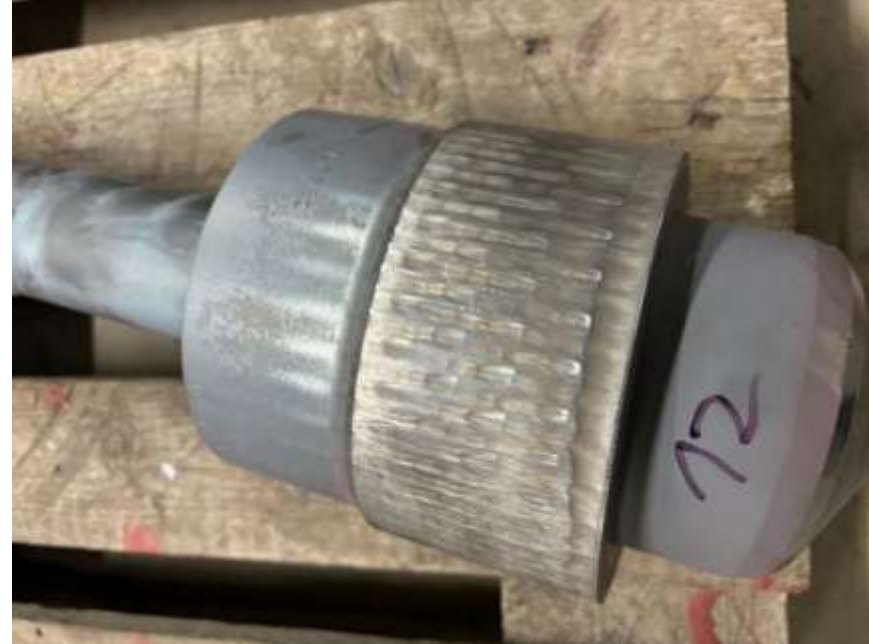
Wear and tear at a HP bypass valve; source: vgbe member company
