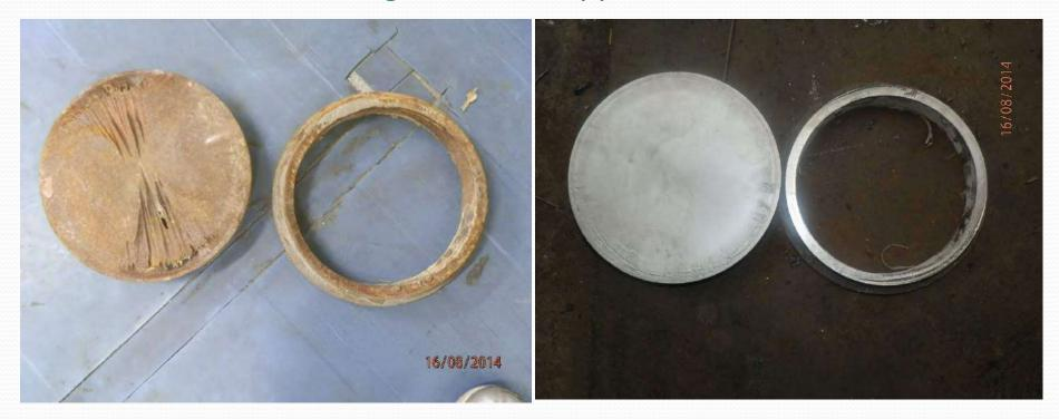
Improved material ASTM A532 Gr.III with hardness >500 BHN.
