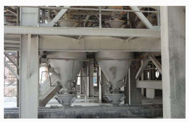
Change in Metallurgy of vacuum pump cone to SS-410.
