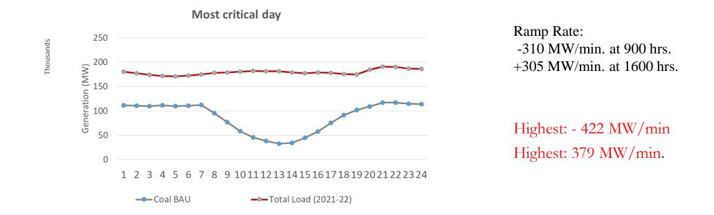
With increase in grid ramping requirements over the years, most of the additional ramping is being met by thermal generation, thermal ramp touched 250 MW/min.
