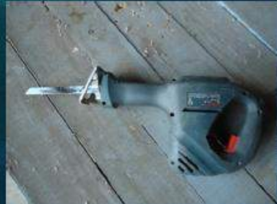
Saber Saw for cutting of tube & fins
