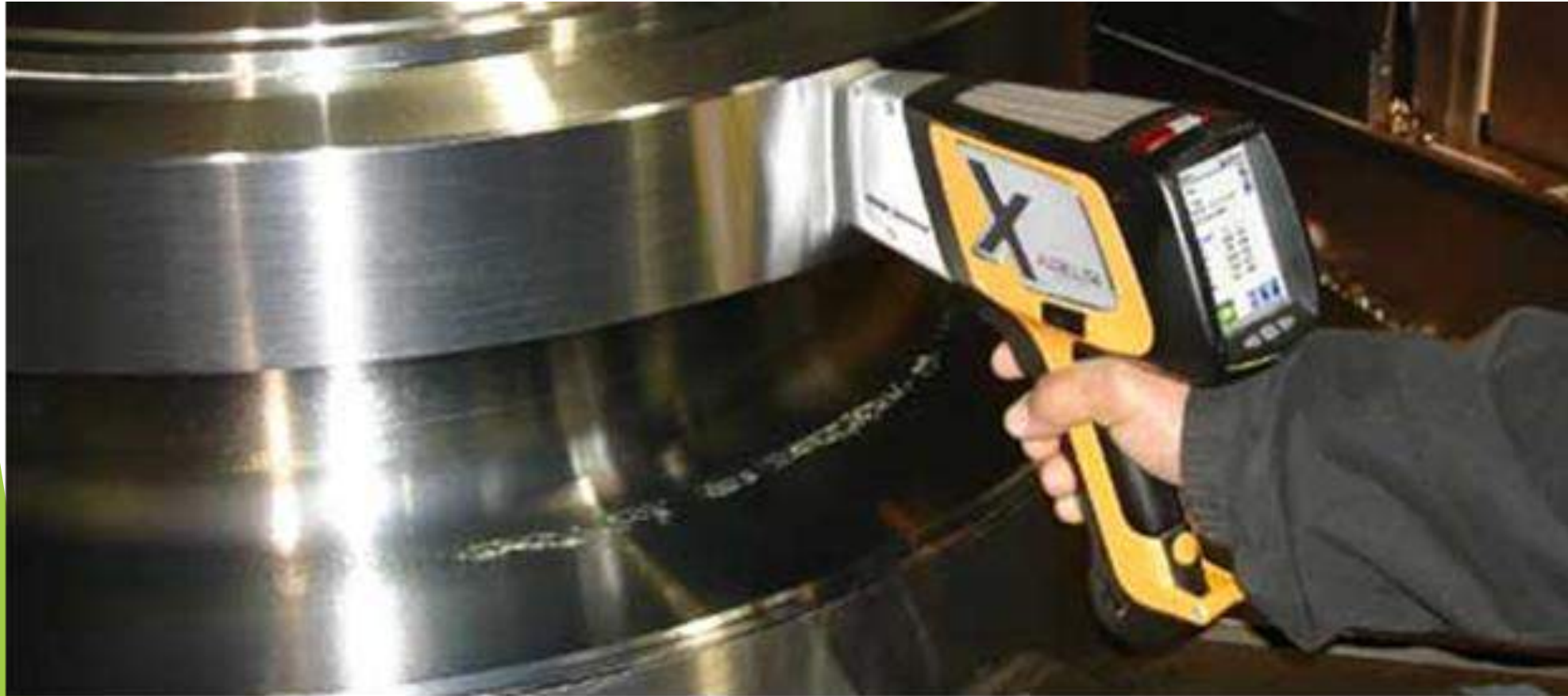
XRF Analyzer for Identifying Material Composition of Spares
