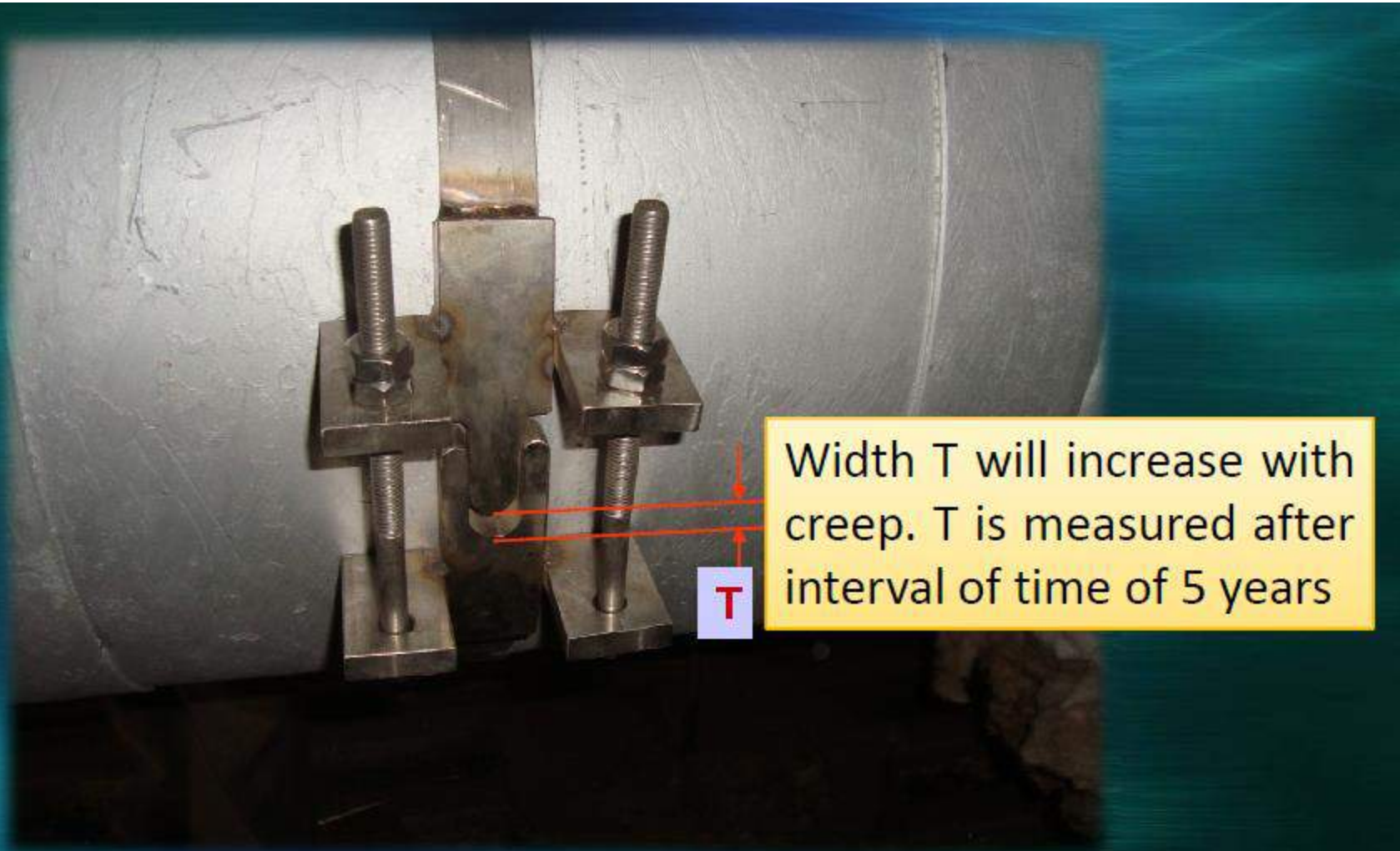
Creep Growth Strain Gauge for tracking of creep in M.S. and R.H. critical piping
