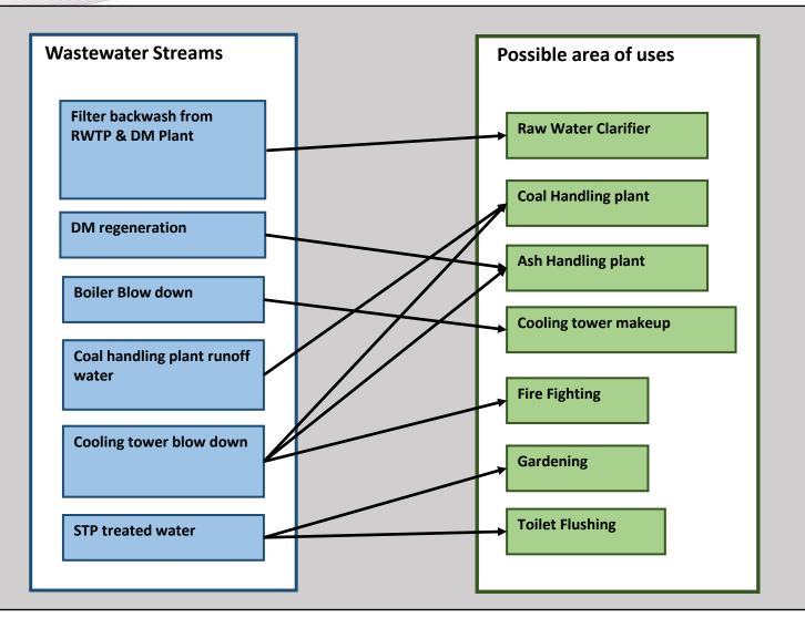
The cooling tower blowdown quantity and the Sewage can be treated up to tertiary level for its utilization in the cooling tower makeup and other low-end applications inside the plant
