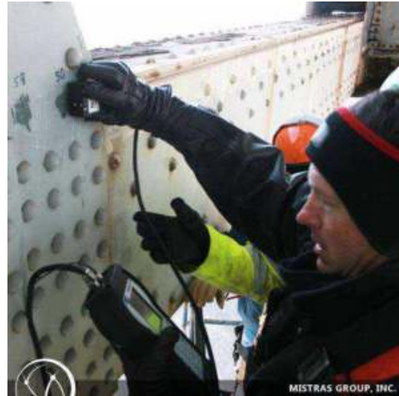
UT Testing for Corrosion
