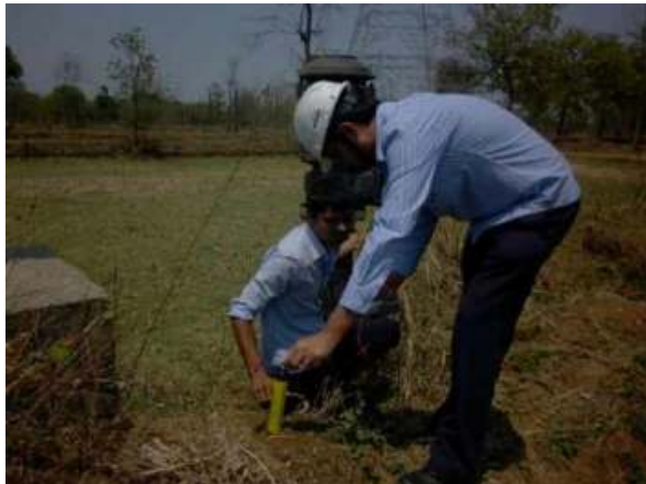
Pipe to soil potential measurement
