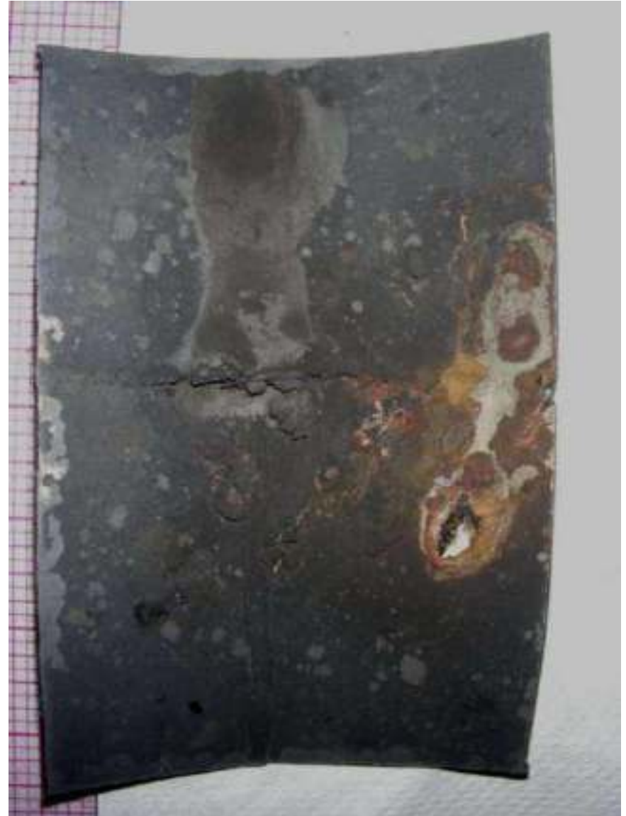
Pitting corrosion – small and large
