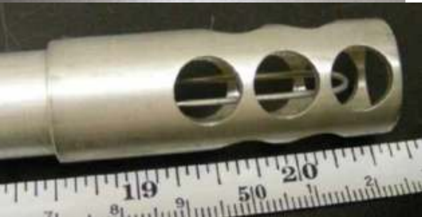
Electrical Resistance Probes
