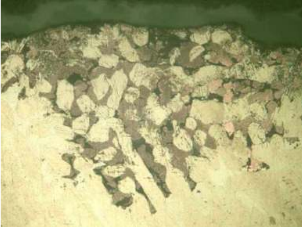
Brass River Water Impellor suffering from dealloying and cavitation
