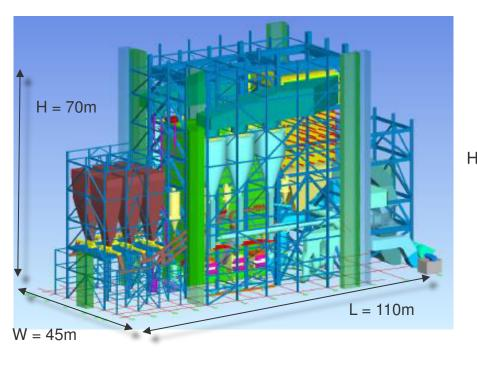
600MW USC PC Boiler (Indonesian Subbituminous) Footprint = 5440m<sup>2</sup> includes FGD@ 900m<sup>2</sup> (Based on Dongbu Green 2x580MW)
