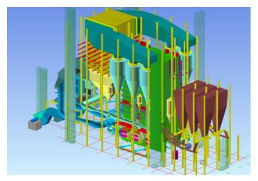
Modularized 2 cyclone model to be adapted to 4 cyclone model
