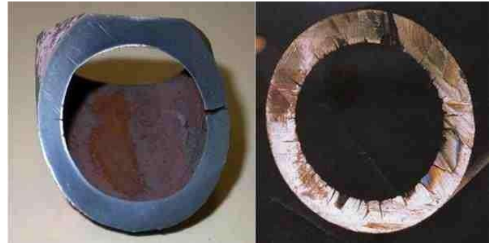
Stress corrosion crack failure
