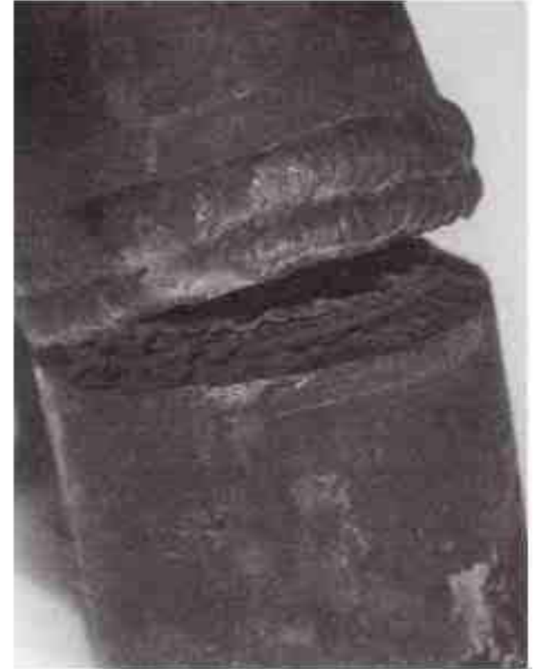
Dissimilar metal weld failure
