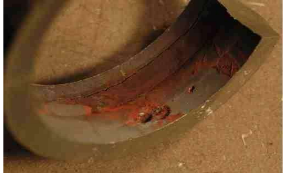
Stress corrosion crack failure
