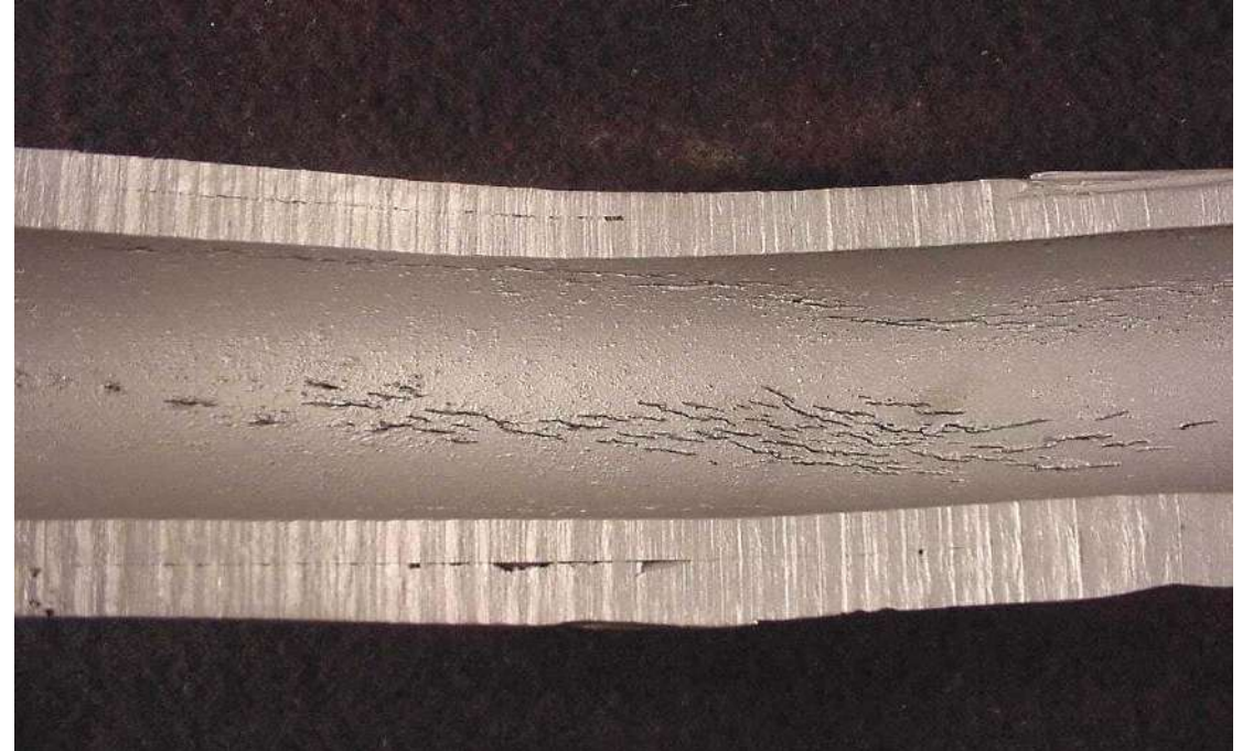
Corrosion fatigue Boiler tube failure
