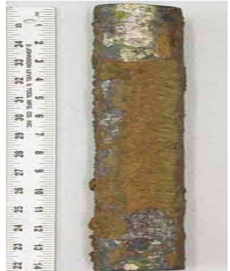
Fire side fuel ash corrosion failure
