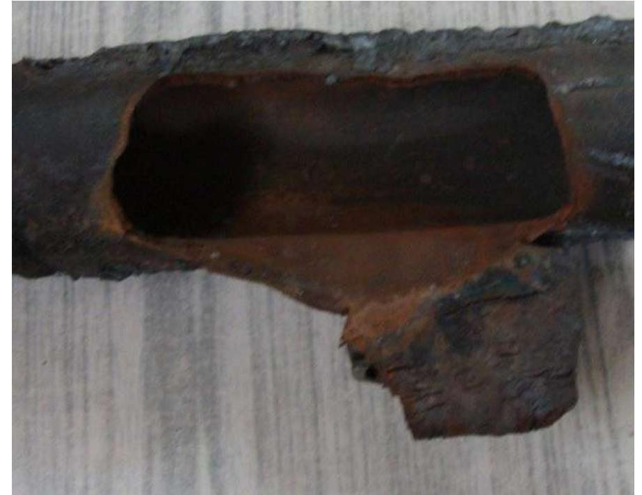
Pictorial view of Boiler tube failure
