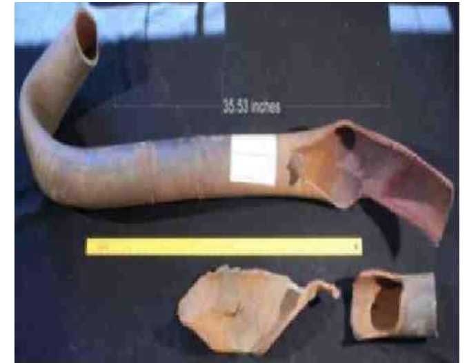
Pictorial view of Boiler tube failure
