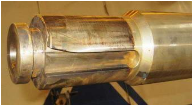
DAMAGED KEY WAY
