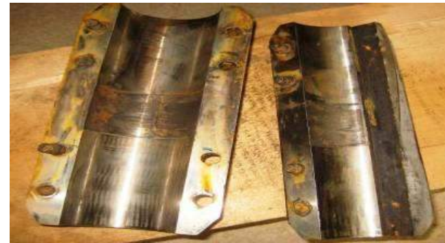
DAMAGED MUFF COUPLING OF CEP
